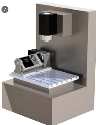
4 th + 5 th axis, 2-spindle, Y-mounting (crosswise)
