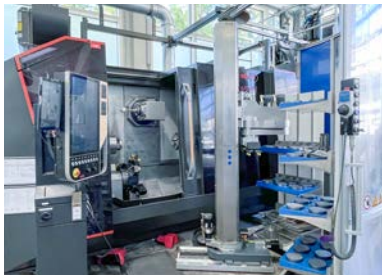
With workpiece pool for unmanned production
