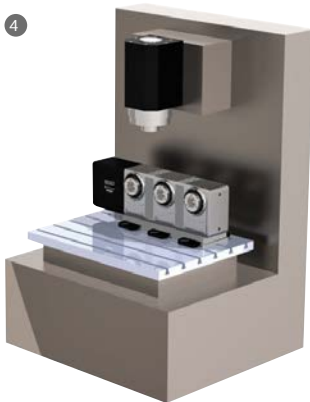
4 th axis, 3-spindle, X-mounting (lengthwise)
