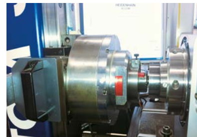
Measuring the indexing accuracy – fully automatically
