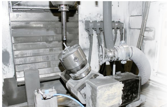
T1-507510 with additional labyrinth seal
