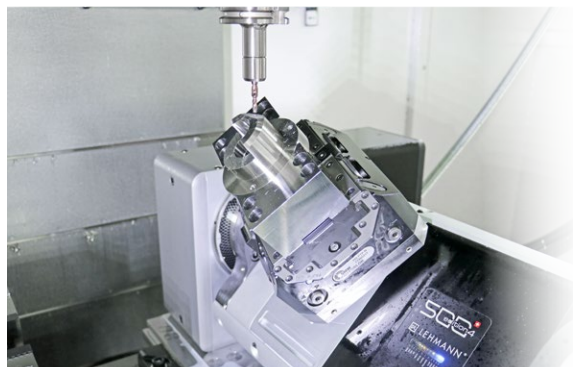
T1-510520 with SCHUNK centric clamping device and a lot of space for much more
