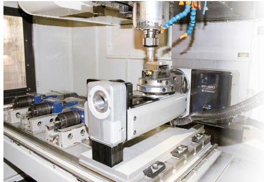
T1-520520 mounted crosswise at the right, leaving a lot of space for other machining
