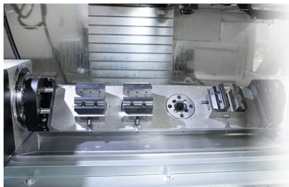
EA-530 with clamping yoke and integrated gredoc zero point clamping system
