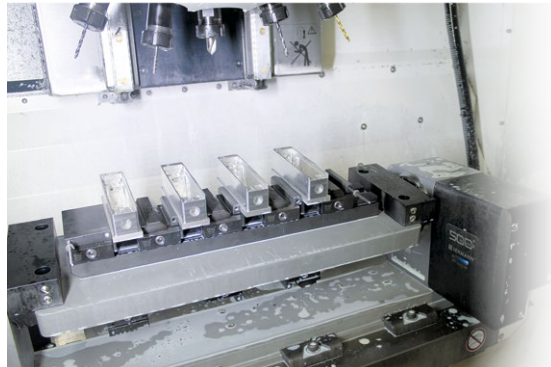
EA-510 rotoFIX clamping yoke, equipped with a rail clamping system
