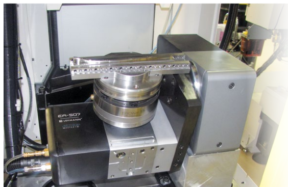
TF-507510 in a special design, with automatic EROWA palletizing
