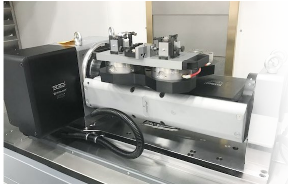
T1-520530 with zero point clamping at 4 locations
