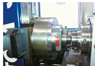
Measuring the indexing accuracy – fully automatically
