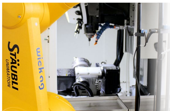
TF-510510 with automatic workpiece clamping
