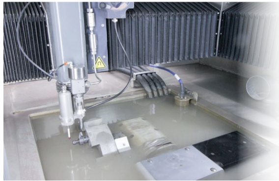
T1-510520 IP68, completely immersed in water bath
