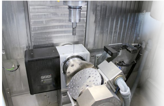
EA-520 as tilting axis; Dividing axis built in-house
