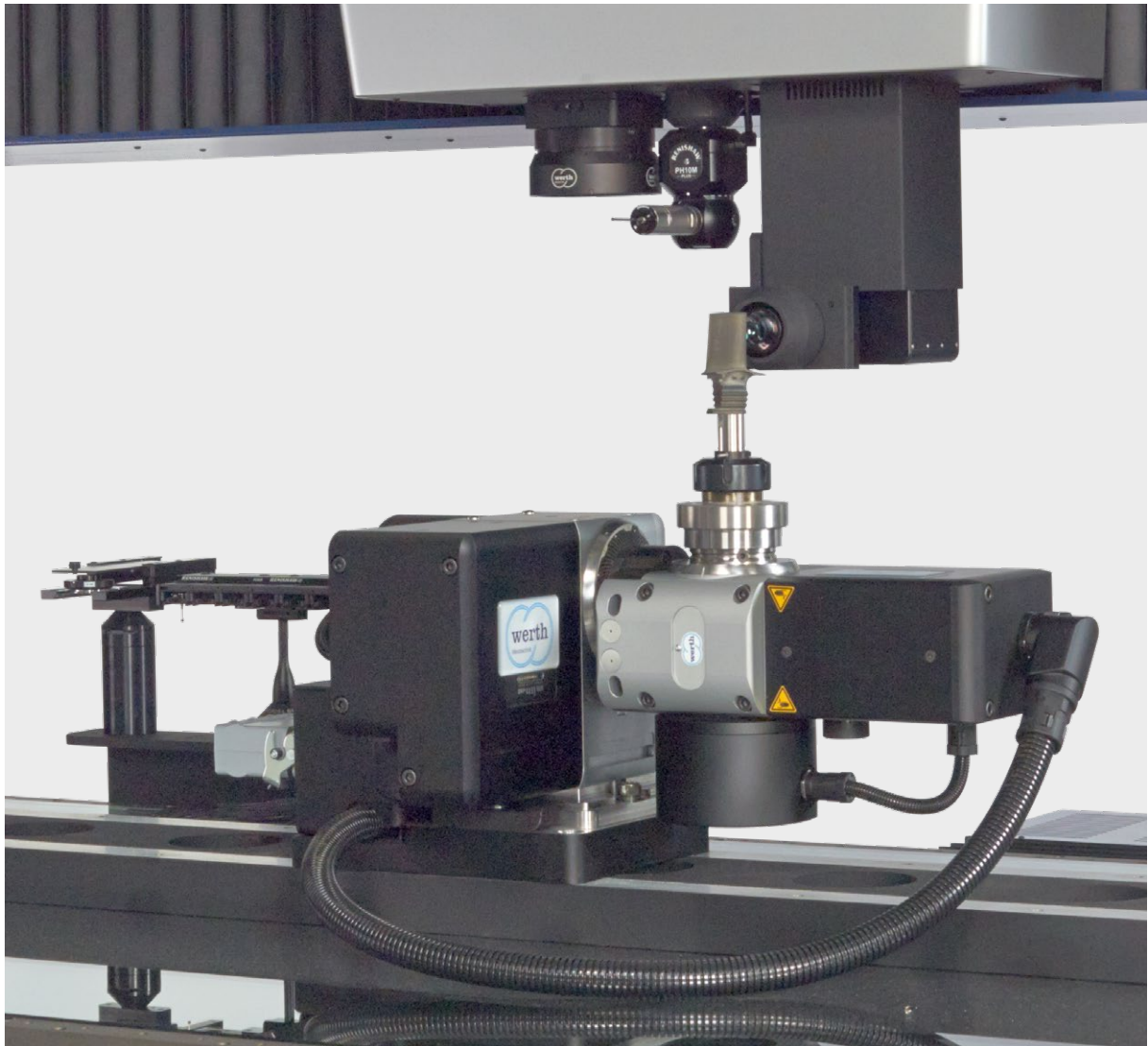
TF-M07M10 on a WERTH Scope-Check in use for measuring a turbine blade
