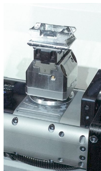
Clamping device automation with HSK ripas adapter. Very compact with high repeat accuracy.
