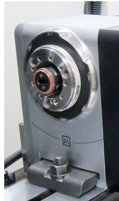
Clamping device automation with HSK ripas adapter. Very compact with high repeat accuracy.
